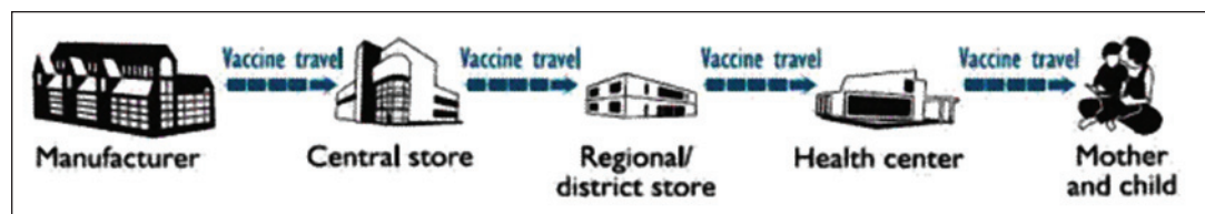
Figure 1. The vaccine cold chain. The last step, from local health center to the recipient, is the most vulnerable (adapted from WHO/PATH documents).
